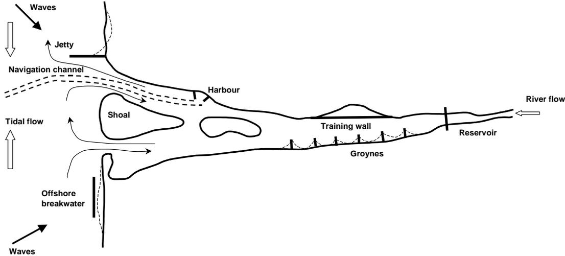
**Fig. 1** Examples of Man-Made Structures in River, Eastuary and Coastal Systems
