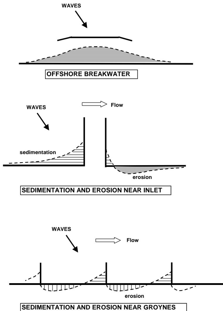
**Fig. 7** Shoreline accretion and erosion near coastal structures (plan view)
