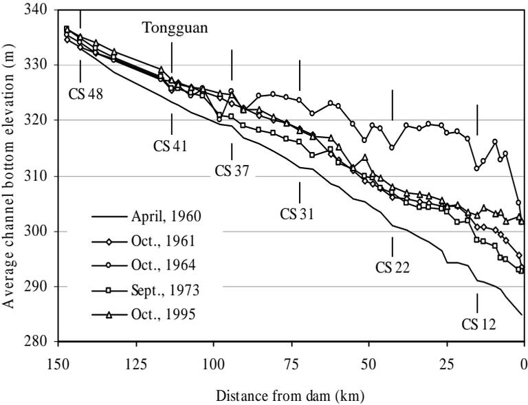
**Fig. 2** Longitudinal Profiles at the Sanmenxia Reservoir During Different Periods of Operation (in which CS12-CS48 are the Measurement Cross Sections on the Reservoir Reach of the Yellow River)
