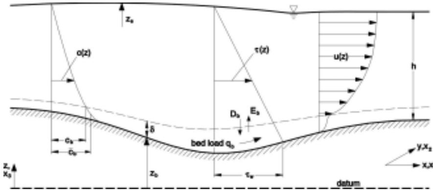
**Fig. 1** Configuration of Flow and Sediment Transport
