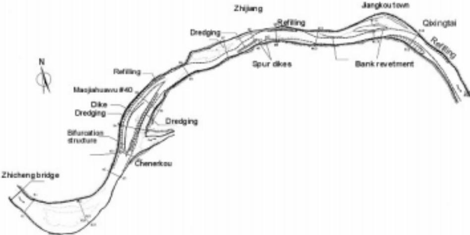
**Fig. 4** Scheme of Channel Improvement in the Zhicheng-Jiangkou Reach
